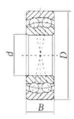
25 mm x 62 mm x 17 mm Loyal 1305 self aligning ball bearings
